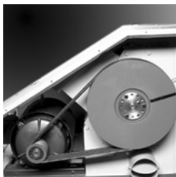
Heavy solid flywheel for added inertia
